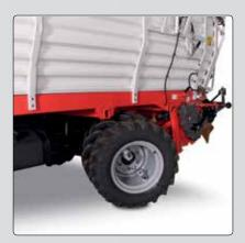
The REFORM PrimAlpin allows the use of the REFORM Muli's **4 wheel steering** as standard. Narrow passages such as farm entrances are thus easily passable. Development focused primarily on a compact design, close to the axle.
