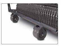
Optimum **ground adjustment** of the pickup is achieved by two support wheels and an optimised pickup suspension.
