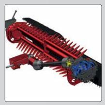
The REFORM PrimAlpin has the tried and tested REFORM quick coupling and is the first built-on self-loading trailer where the **conveyor unit** is driven by a gear unit. It thus excels with particularly smooth operation and minimum maintenance. The closed design also protects the gear unit better against soiling.
