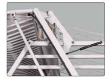
By an innovative concept, the cross tube is raised along with the **tailgate**. This enlarges the opening, and the crop can be unloaded without a bottleneck. This will save valuable time.
